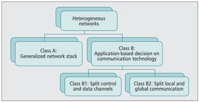
Figure 3. Classification of heterogeneous vehicular networking approaches.
