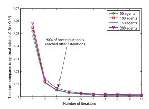
Figure 3: Reduction of total cost over the course of the algorithm for different agent populations sizes.
